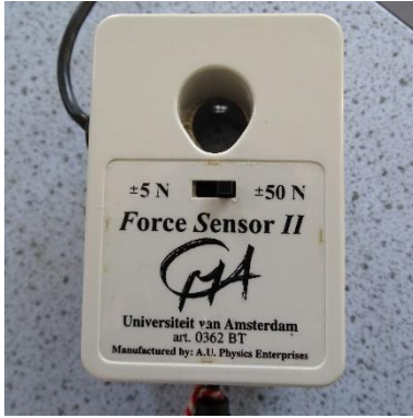
Fig 3: CMA Force Sensor II
