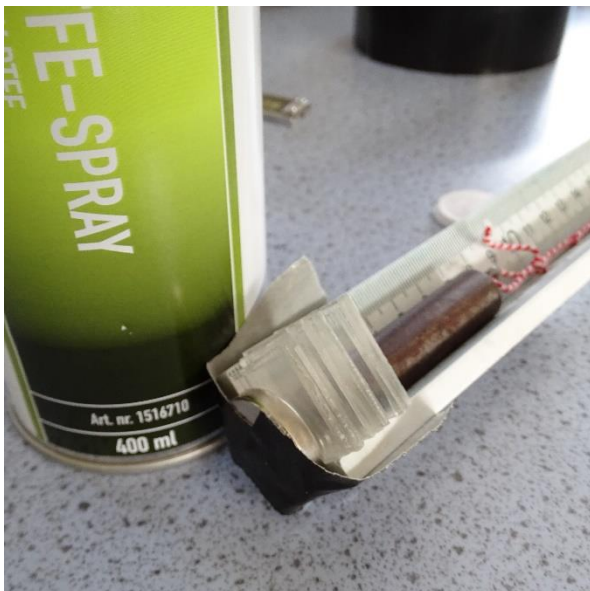
Fig 1: Neodymium magnet taped to head end
